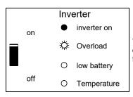
The nominal output of the inverter is exceeded. The "overload" LED flashes.
