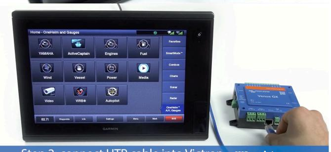
Step 2: connect UTP cable into Victron
