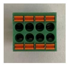
The two on the left are digital input one (open or short them), the next two are digital input 2, and-so-forth. Where upper row is signal and lower row is GND for all four inputs.
