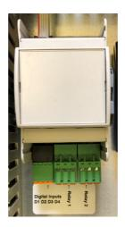
For both, the connector can be pulled free for easy wiring, and then re-insterted.
